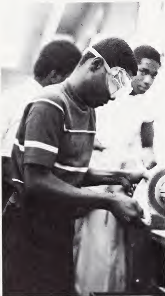
EMMITT PERKINS polishes an aluminum ash tray casting on the wire burnishing wheel, being supervised by Gerald Murray, while Larry Alexander and Tony Radford wait their turn at the machine.
